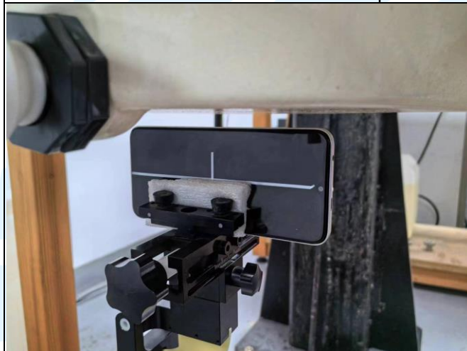
Left Side of EUT with 1.0 cm Gap
