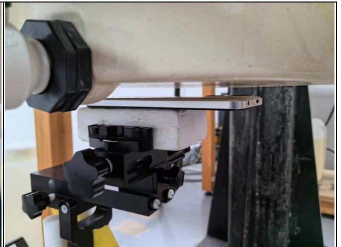
Rear Face of EUT with 1.0 cm Gap
