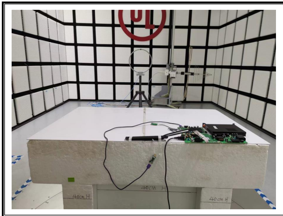
RADIATED RF MEASUREMENT SETUP (Below 30MHz)
