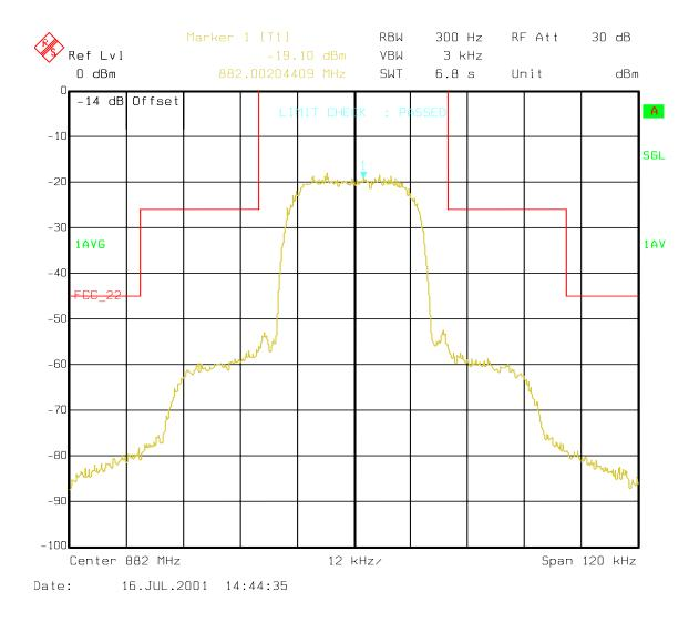
Mid Cellular Frequency Band: Channel 400, 882.00 MHz Measured at the output of SBEDRU transceiver, backplane terminal
