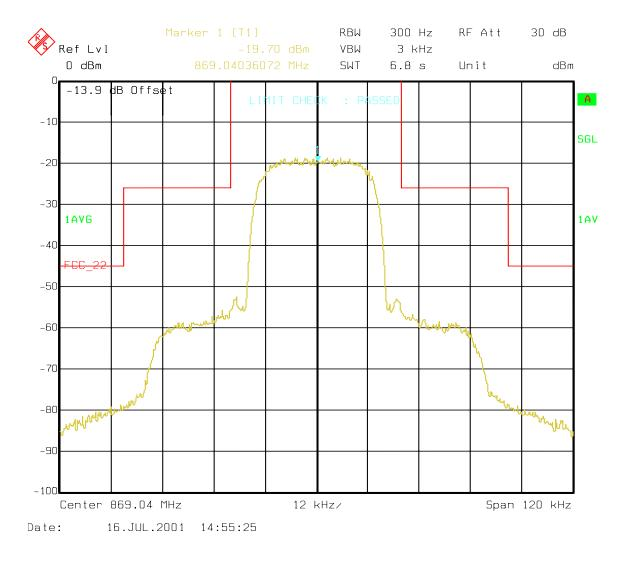
Cellular A-Band: Lower Edge Channel Channel 991, 869.04 MHz Measured at the output of SBEDRU transceiver, backplane terminal
