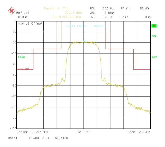
Cellular B-Band: Upper Edge Channel Channel 799, 893.97 MHz Measured at the output of SBEDRU transceiver, backplane terminal
