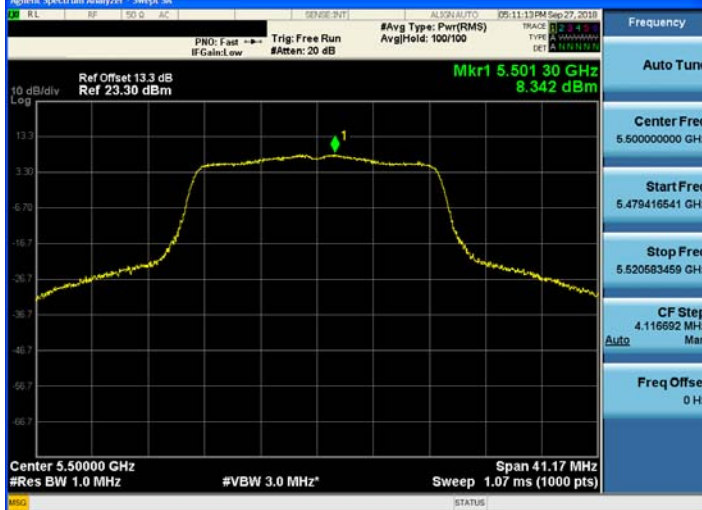
802.11ac_VHT20 UNII 2C BAND PSD CH 100
