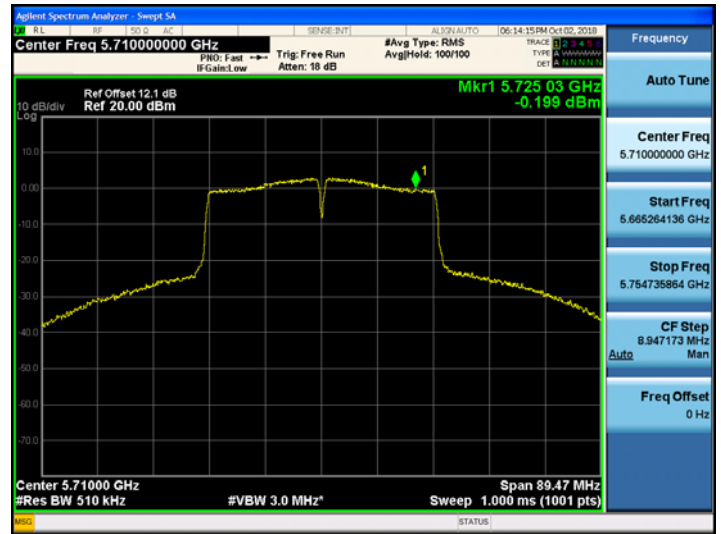
802.11ac_VHT40 UNII 3 Band PSD CH.142
