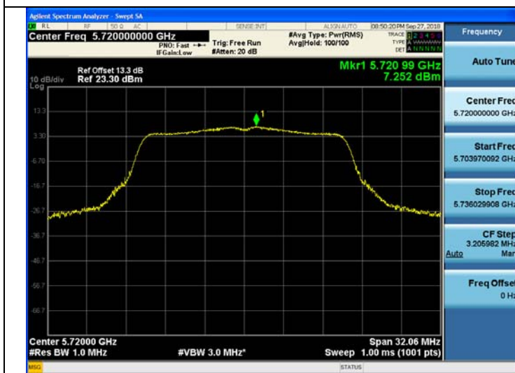
802.11n_HT20 UNII 2C Band PSD CH.144
