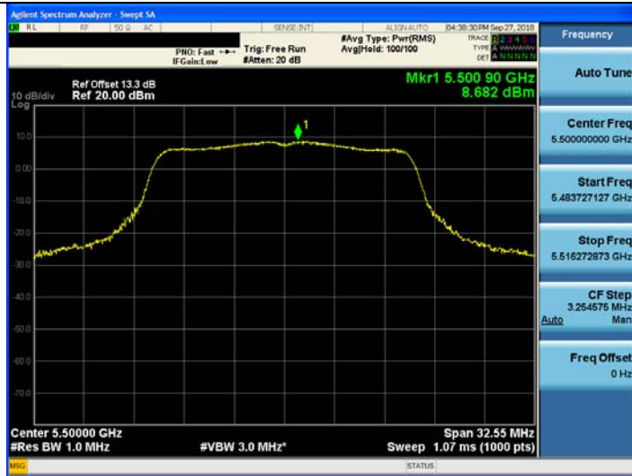
802.11a UNII 2C BAND PSD CH 100
