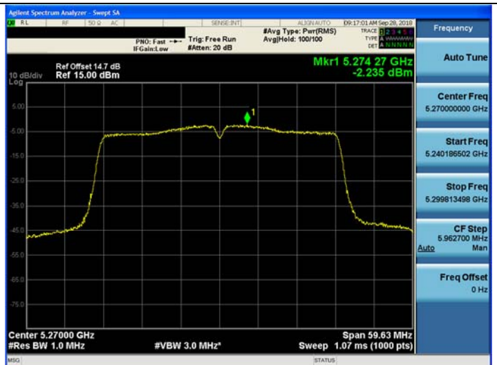
802.11ac_VHT40 UNII 2A BAND PSD CH 54_External Ant
