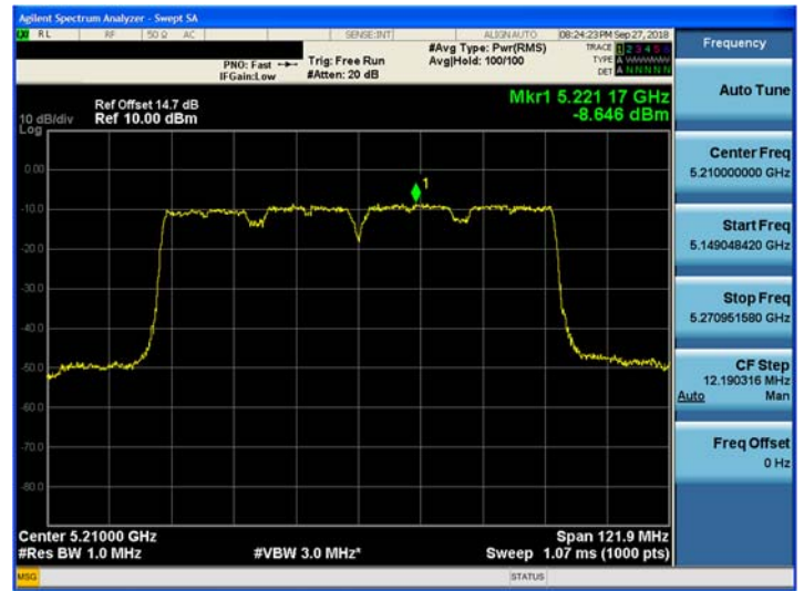
802.11ac_VHT80 UNII 2A BAND PSD CH 58_External Ant
