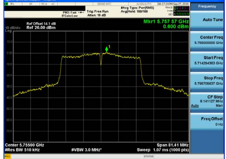
802.11ac_VHT40 UNII 3 BAND PSD CH 151
