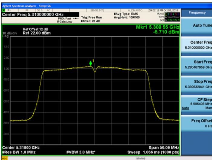
802.11ac_VHT40 UNII 2A BAND PSD CH 62_Internal Ant
