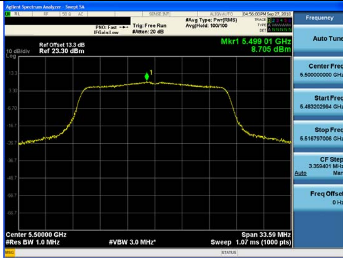
802.11n_HT20 UNII 2C BAND PSD CH 100
