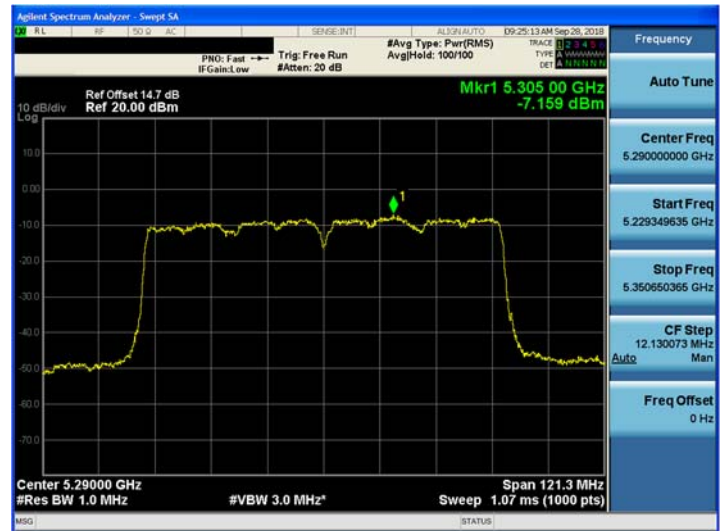
802.11ac_VHT80 UNII 2A BAND PSD CH 58_External Ant
