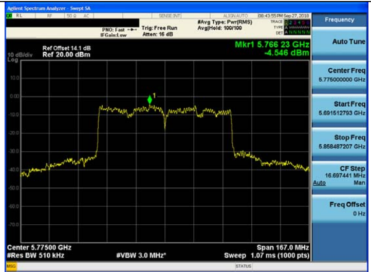
802.11ac_VHT80 UNII 3 BAND PSD CH 155
