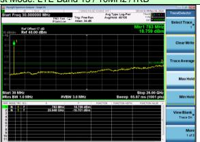
Test Mode: LTE Band 13 / 10MHz /50RB
