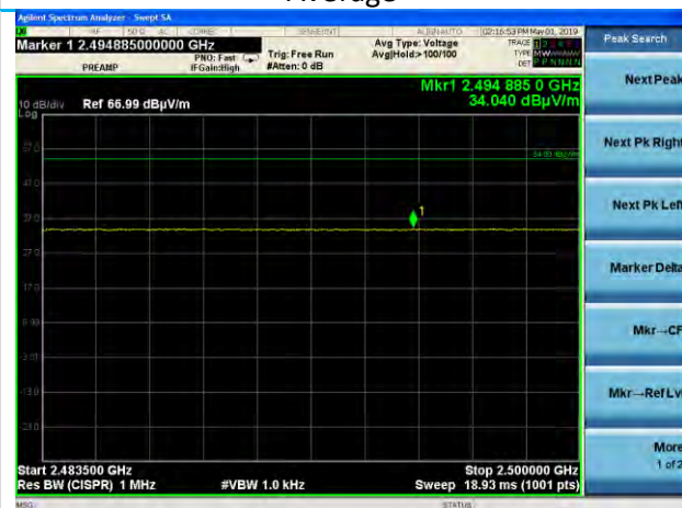
2483.5-2500 MHz, EUT Flat, EDR2, High Channel Average
