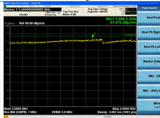
2500-4000 MHz, GFSK, Low Channel, Horizontal Antenna, Peak with Average Limit
