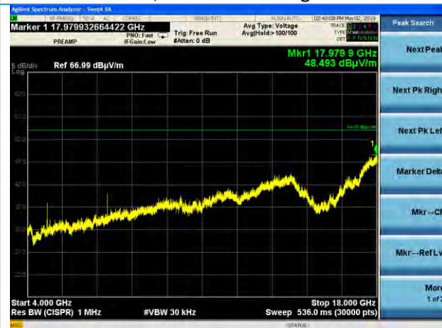
4-18 GHz, GFSK, Low Channel, Horizontal Antenna, Peak with Average Limit, Flat EUT
