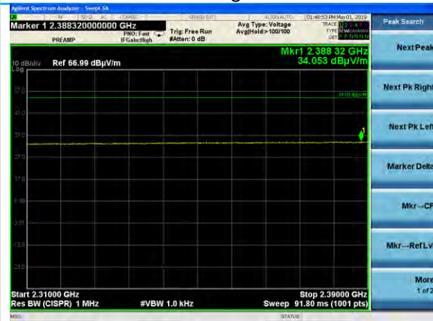
2310-2390 MHz, EUT Flat, EDR3, Low Channel Average
