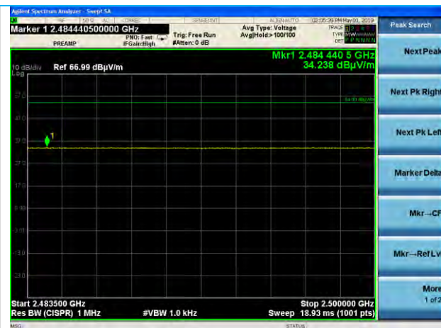
2483.5-2500 MHz, EUT Flat, GFSK, High Channel Average
