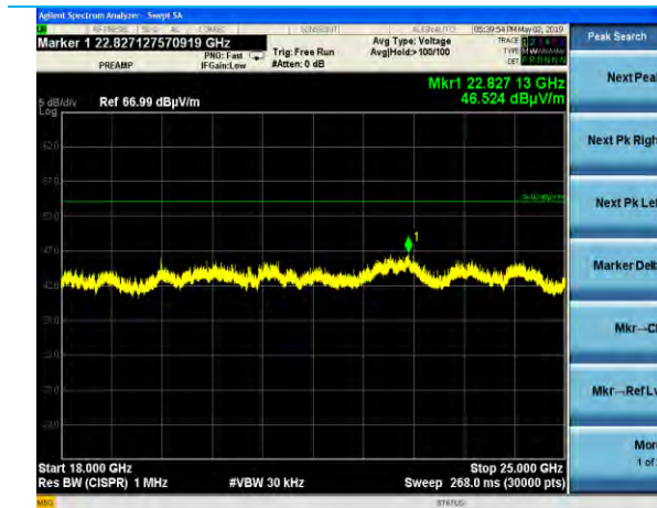
18-25 GHz, GFSK, Low Channel, Vertical Antenna, Peak with Average Limit, Flat EUT
