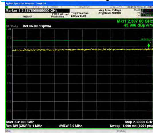
2310-2390 MHz, EUT Flat, EDR3, Low Channel Peak with Average Limit
