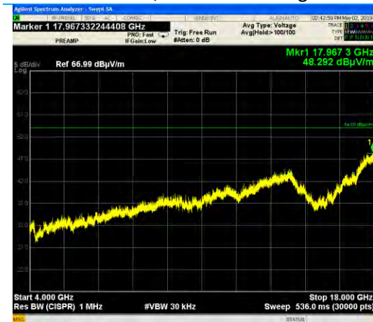
4-18 GHz, GFSK, Low Channel, Vertical Antenna, Peak with Average Limit, Flat EUT
