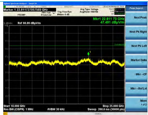
18-25 GHz, GFSK, Low Channel, Horizontal Antenna, Peak with Average Limit, Flat EUT
