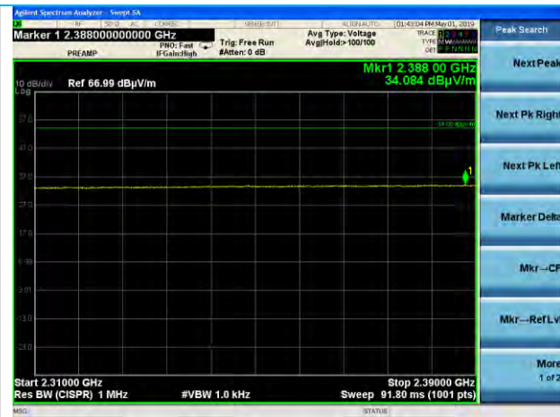
2310-2390 MHz, EUT Flat, EDR2, Low Channel Average
