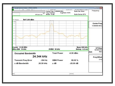
Note: Because the measured signal is CW or CW-like, adjusting the RBW per C63.10 would not be practical since the measured bandwidth will always follow the RBW.
