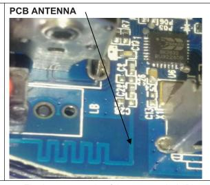
The antenna is integral antenna. The best case gain of the antenna is 0dBi.
