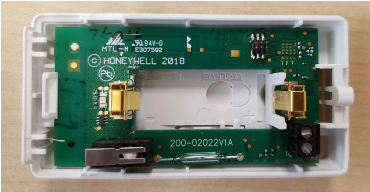
CASE INTERIOR WITH PCB INSTALLED
