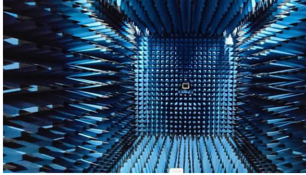
Figure 2: Geometry of Anechoic Chamber for Radiation patterns.
