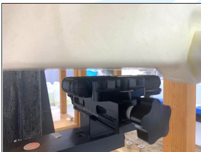
Front Face of EUT with 1.0 cm Gap
