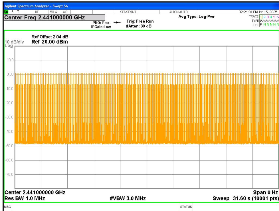
Dwell NVNT 3-DH5 2441MHz Ant1 One Burst
