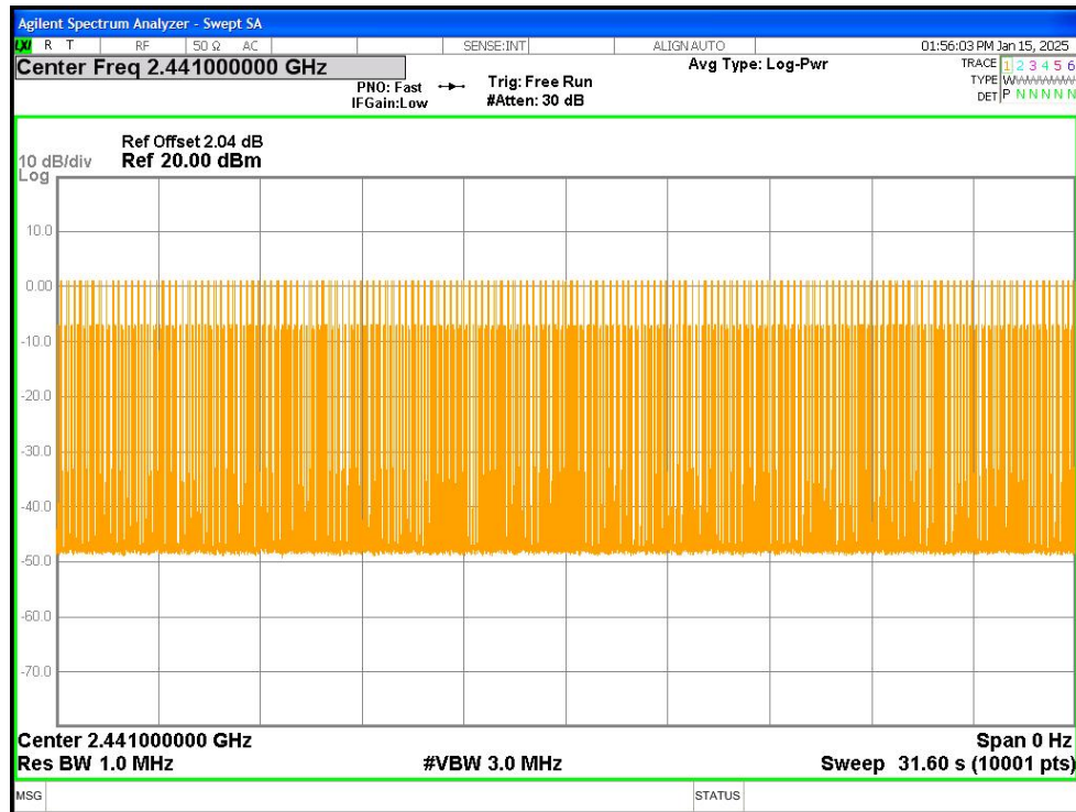
Dwell NVNT 1-DH3 2441MHz Ant1 One Burst
