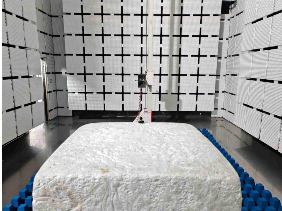
Radiated Emissions (above 1GHz)
