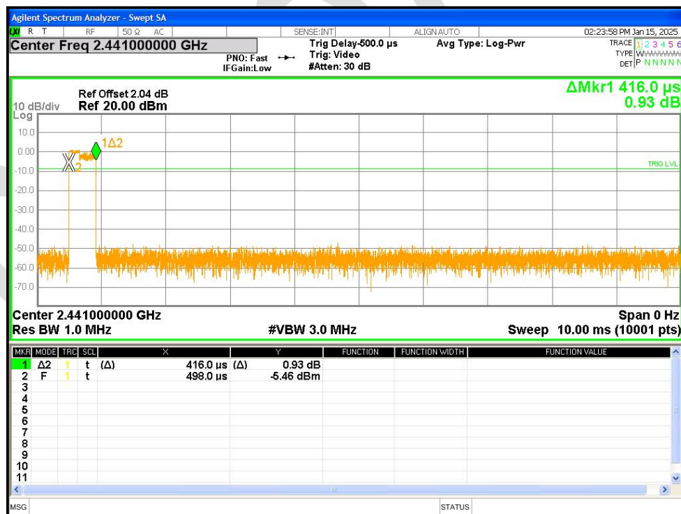
Dwell NVNT 3-DH1 2441MHz Ant1 Accumulated
