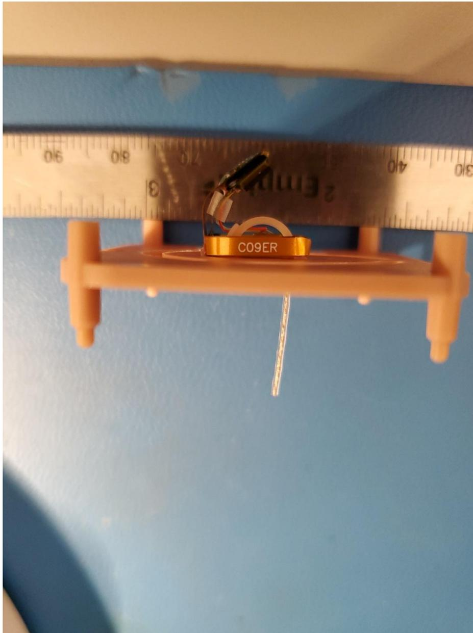
Figure 1 2.4 GHz Antenna (scale in mm)
