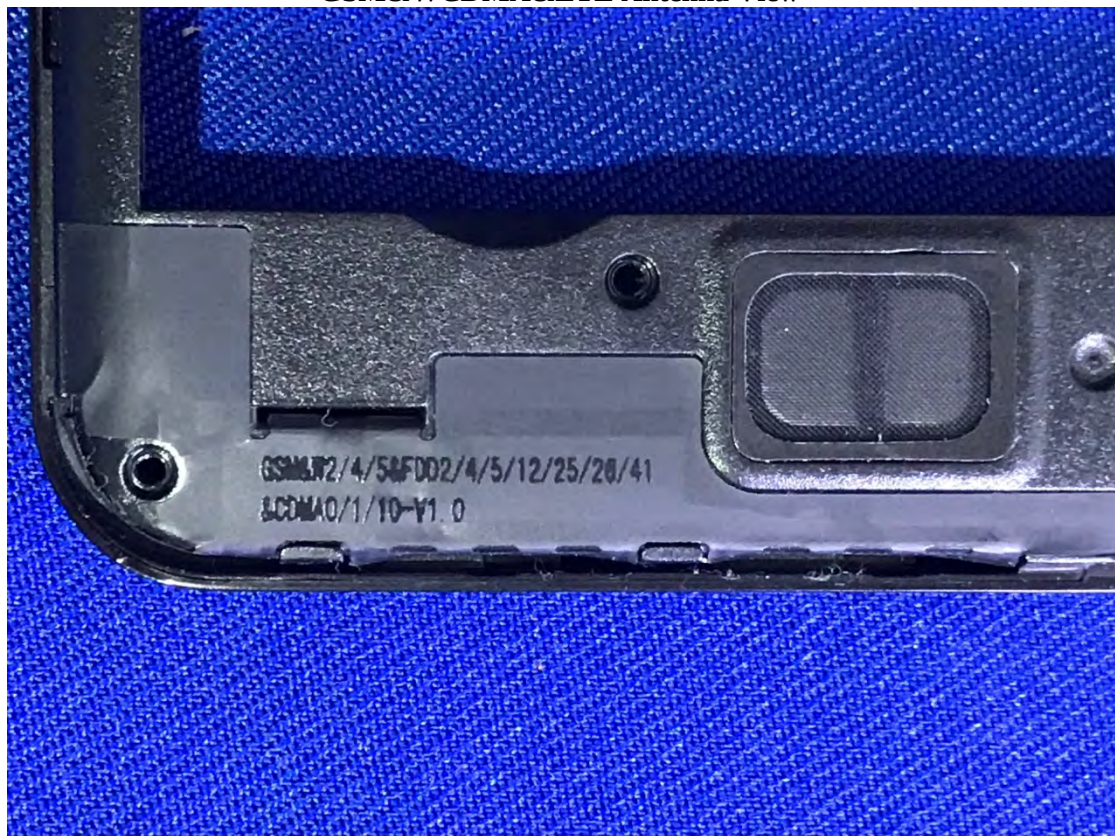
GSM&WCDMA&LTE Antenna View
