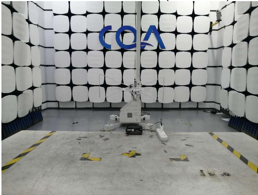
Radiated emission Test Setup (30MHz~1GHz)
