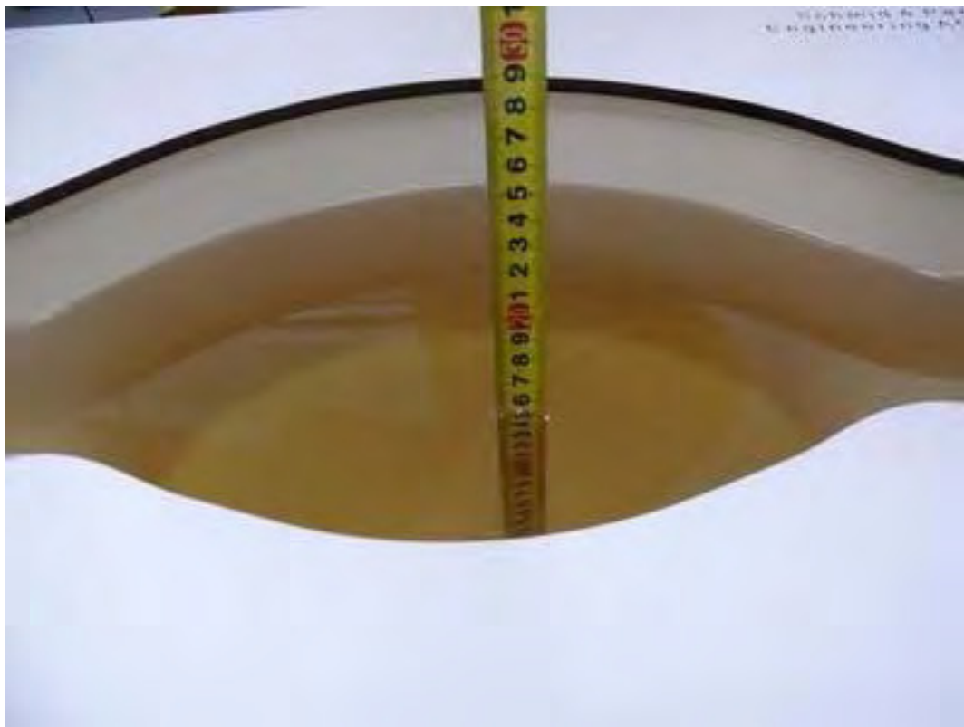
Picture 3: Liquid depth in the flat Phantom (750MHz, 15.4cm depth)
