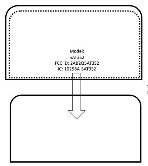
Slide back cover off the device. Label printed on inside of device.
