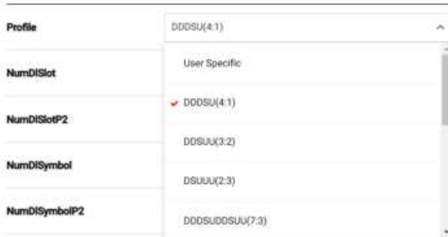
**Figure 42. The Askey 5G NR Small Cell DU Configuration – Time Slot Parameters**
