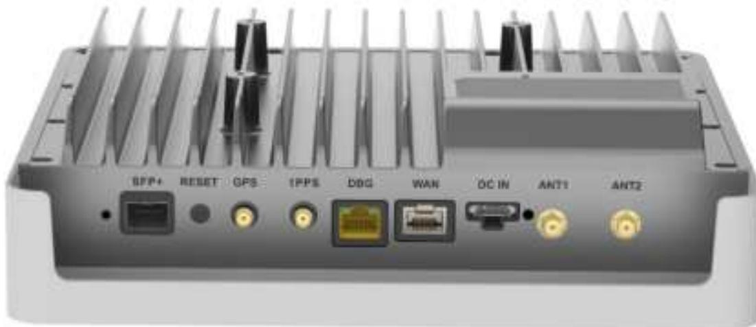
The DBG port is a debug or rescue interface with the default Static IP **192.168.8.100**. You can connect directly to a PC/NB and surf the Admin Web by the URL **http://192.168.8.100** on PC/NB. The network setting of the DBG port could be modified if surfing the Admin Web by the method. But it only supports the Static IP mode starting with **192.168.8.** and doesn't support the gateway and name server.
