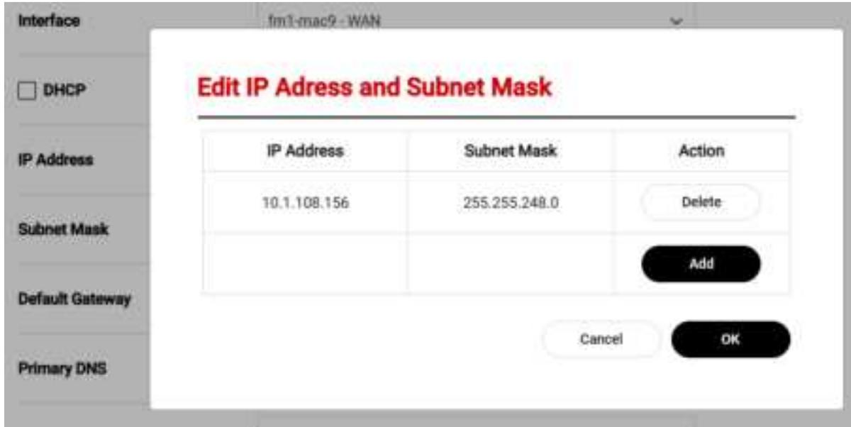
The IP address and subnet mask value can be modified directly on the dialog window, and remove the item by clicking the Delete button. If you want to add a new item, click the Add button and edit the configuration.
