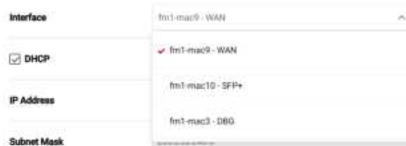
It means that you can click the item to modify the IP address of the DBG interface. As per the above statement, the IP address of the DBG interface only supports static IP starting with 192.168.8. and doesn't support to modify the gateway or name server. The GUI has some differences from other ports, as shown in the following illustration:
