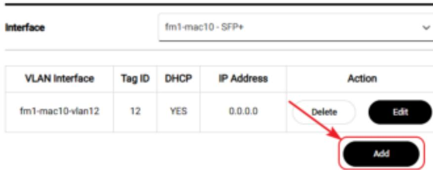
Click the **Add** button will prompt a window to create a new VLAN attached to the physical network interface. The DNS configurations are optional for the VLAN with static IP. If the DHCP is enabled, add the ignore default route option Ignore **Routes**.
