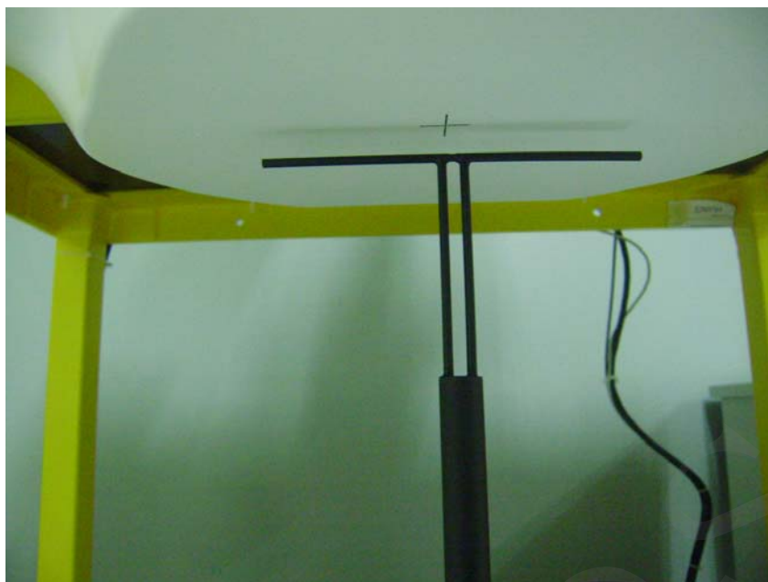
Setup Photo of Dipole Antenna
