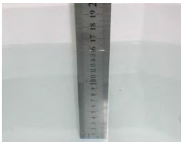
Liquid Height for Head SAR
