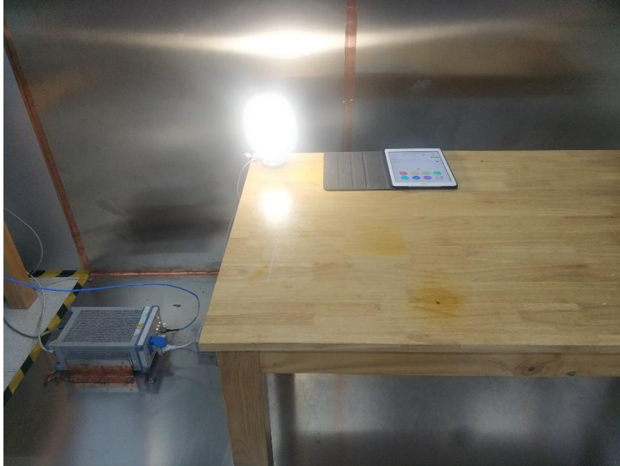
Photograph 6: Set-up for Conducted Emission on AC Mains
