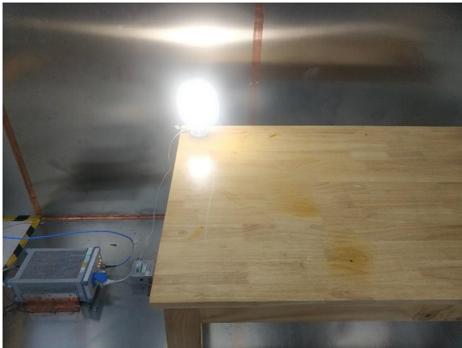
Photograph 6: Set-up for Conducted Emission on AC Mains
