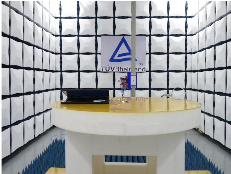
Photograph 3: Set-up for Radiated Spurious Emission, Above 1GHz
