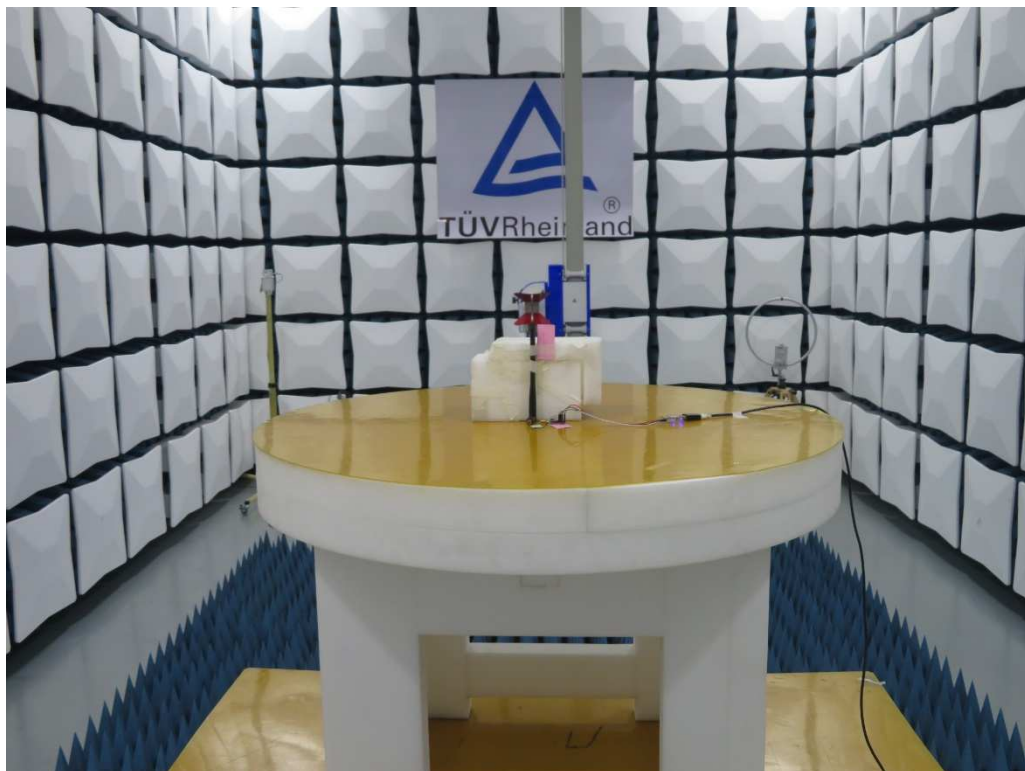
Photograph 2: Set-up for Radiated Spurious Emission, Above 1GHz
