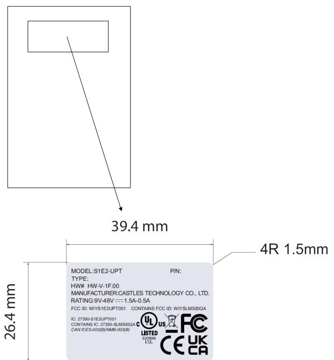
Note: There is no space to bear Part 15.19 statement due to placing the statement on the device cannot be done without ruining the aesthetics, which would impact revenue, the statement is specified in user manual.
