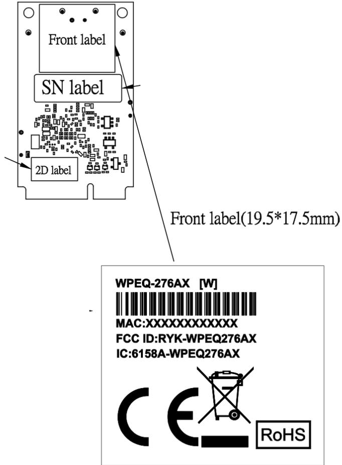
The label shown is permanently affixed at a conspicuous location on the device with a permanent adhesive and be readily visible to the user at the time purchase (Labeling requirements per 2.925).
