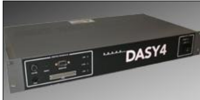
Figure 11: DASY4 measurement server
