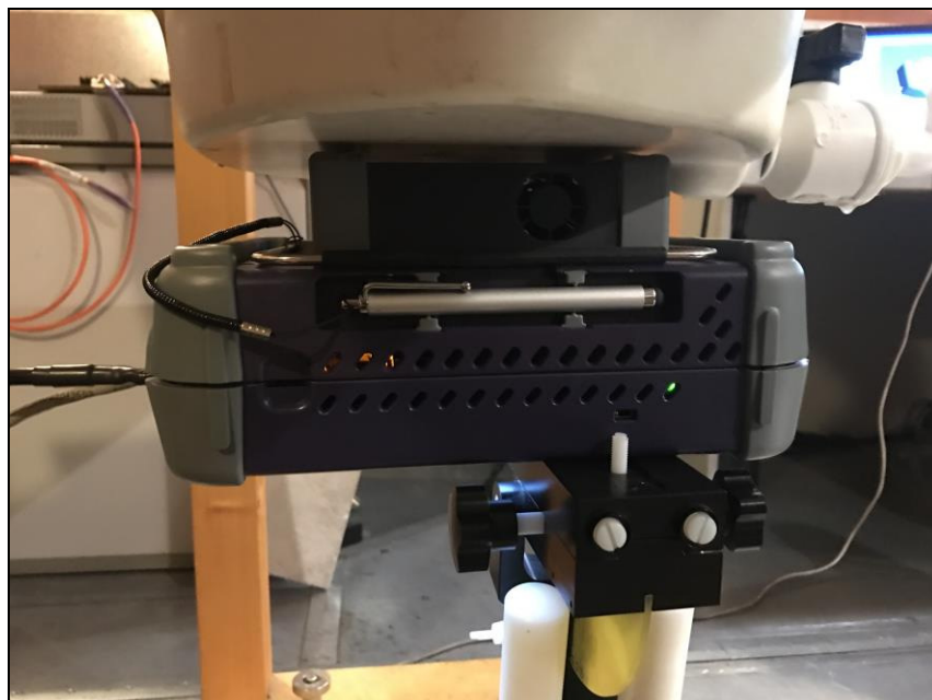
Figure 20: EUT with Back of EUT against Phantom
