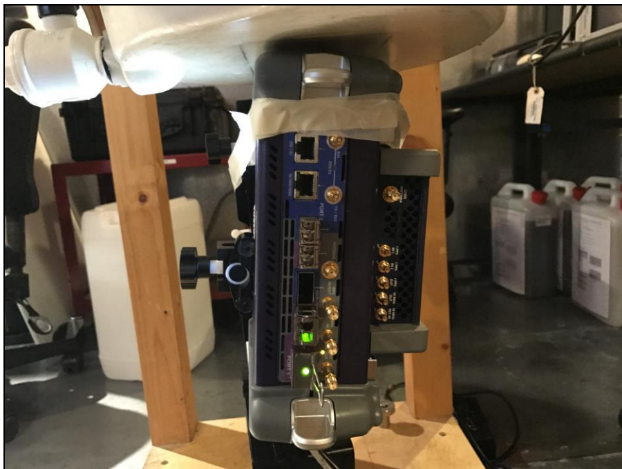
Figure 18: EUT Left Edge, Side against Phantom
