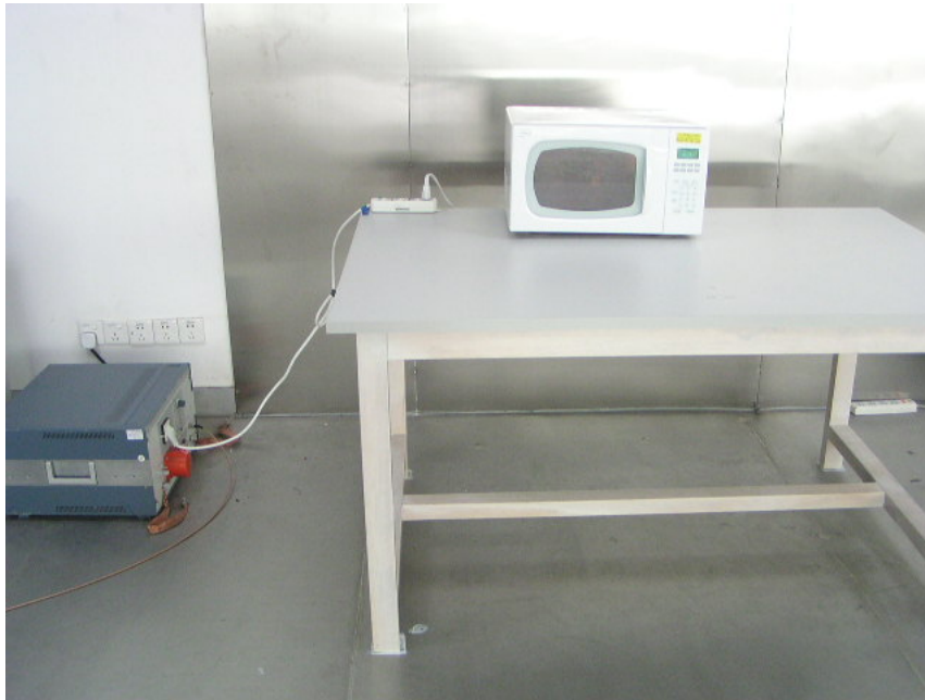
Conducted Emission–Side View
