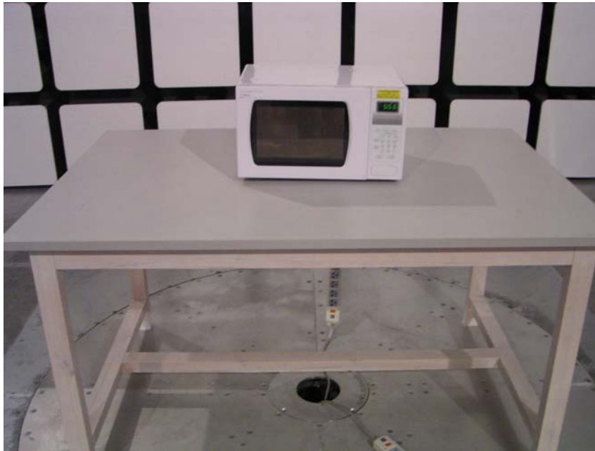
Radiated Emission–Front View (30MHz-1000MHz)
