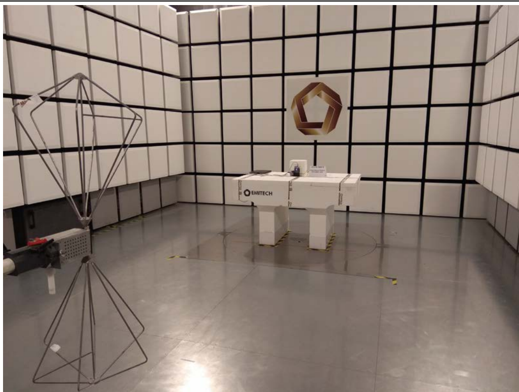
TEST SETUP PHOTO(S) RADIATED EMISSIONS (30MHz-200MHz)
