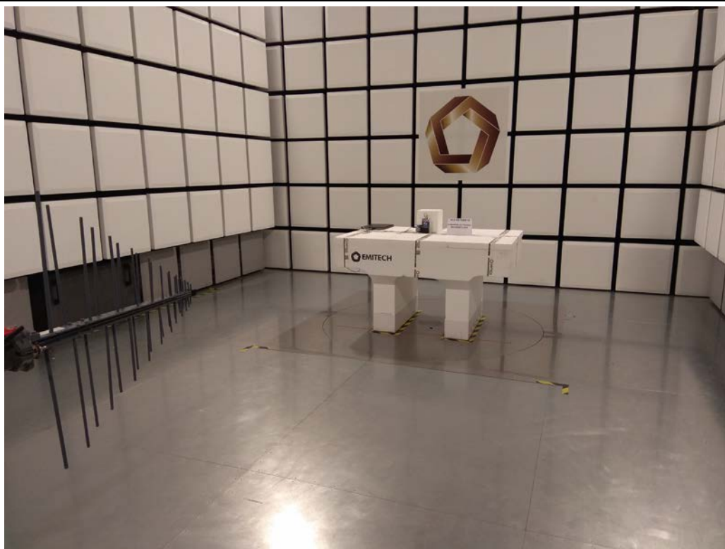
TEST SETUP PHOTO(S) RADIATED EMISSIONS (200MHz-1GHz)
