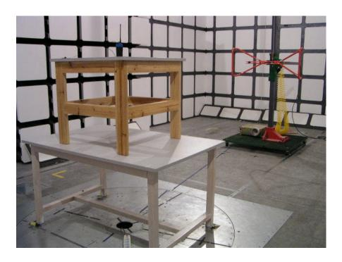
Radiated Emission - Rear View (30-1000 MHz)
