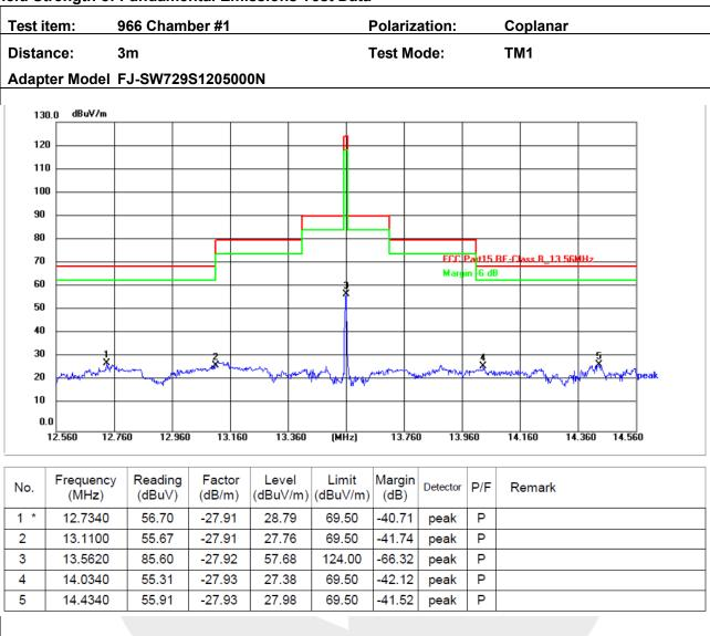
Note: Level = Reading + Factor Margin =Level - Limit
