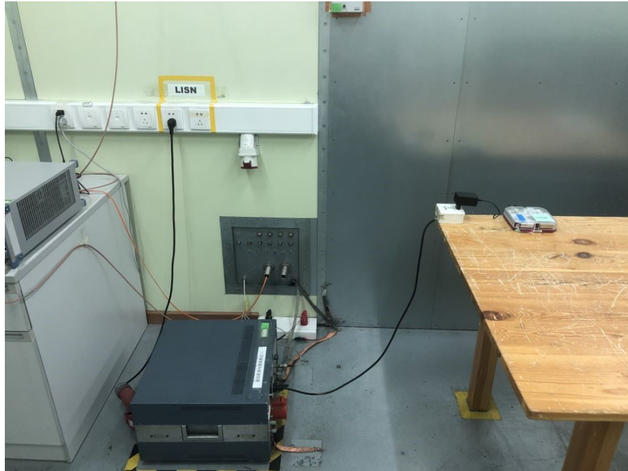
Photograph 3: Set-up for Conducted Emission on AC mains
