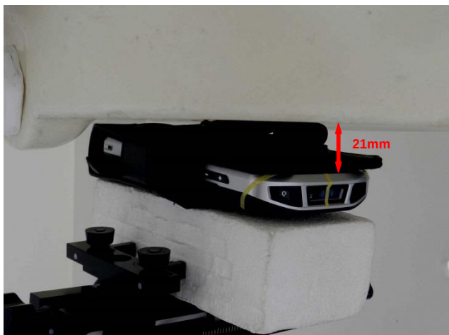
Front with Soft Holster, Test Separation 0 mm
