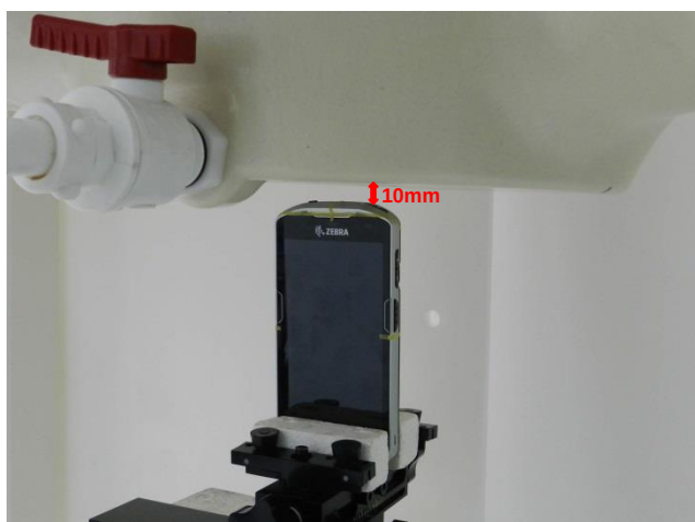
Top Side, Test Separation 10 mm
