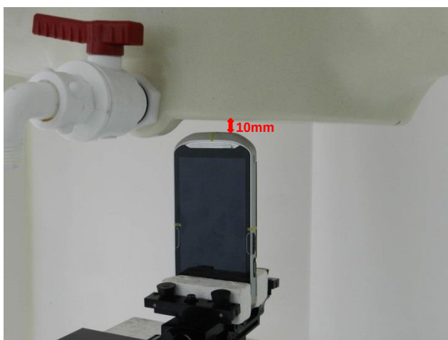
Bottom Side, Test Separation 10 mm
