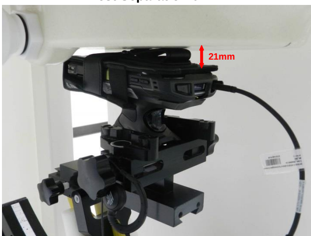
Front with Soft Holster + Exoskeleton + Trigger Handle + 3.5mm Earphone, Test Separation 0 mm
