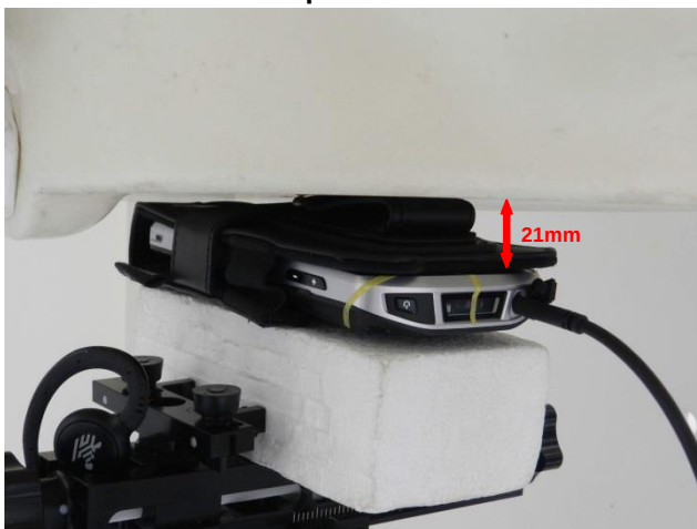
Front with Soft Holster + 3.5mm Earphone, Test Separation 0 mm
