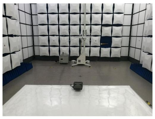
RADIATED EMISSION ABOVE 1G TEST SETUP
