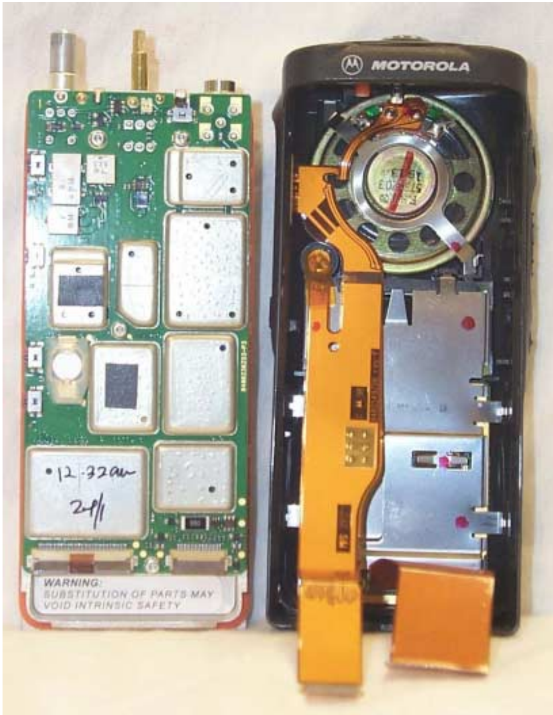
REAR VIEW WITH CIRCUIT BOARD REMOVED FROM HOUSING (MATING SURFACES OF BOARD AND HOUSING ARE SHOWN)
