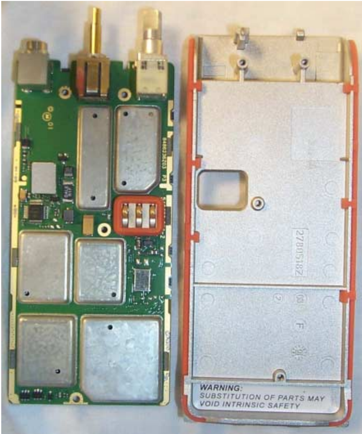
REAR VIEW WITH CIRCUIT BOARD REMOVED FROM CHASSIS (MATING SURFACES OF CIRCUIT BOARD AND CHASSIS ARE SHOWN)
