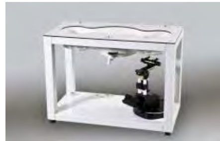
Figure E.5.1 SAM Twin Phantom
