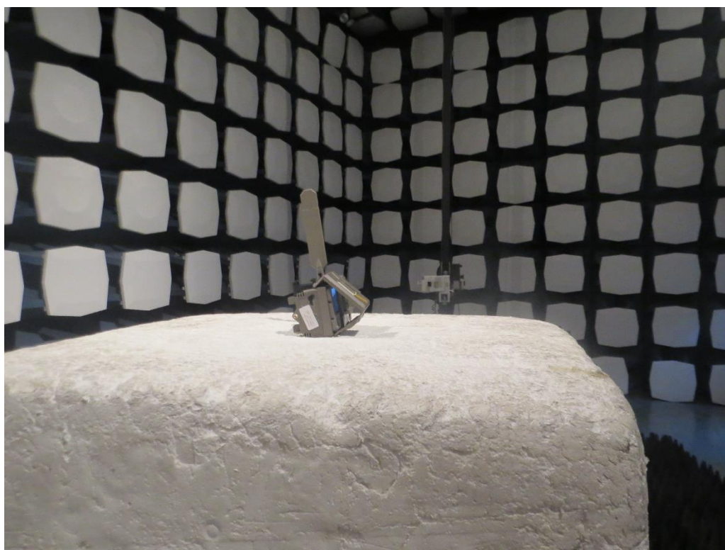
Picture 1 Radiated Emission Test Setup
