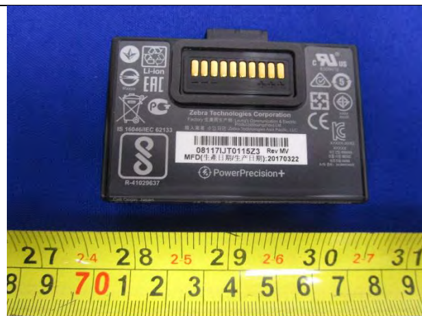
EUT - Battery View
