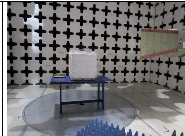
Radiated Emissions (>1GHz) – Front View (EUT horizontal)
