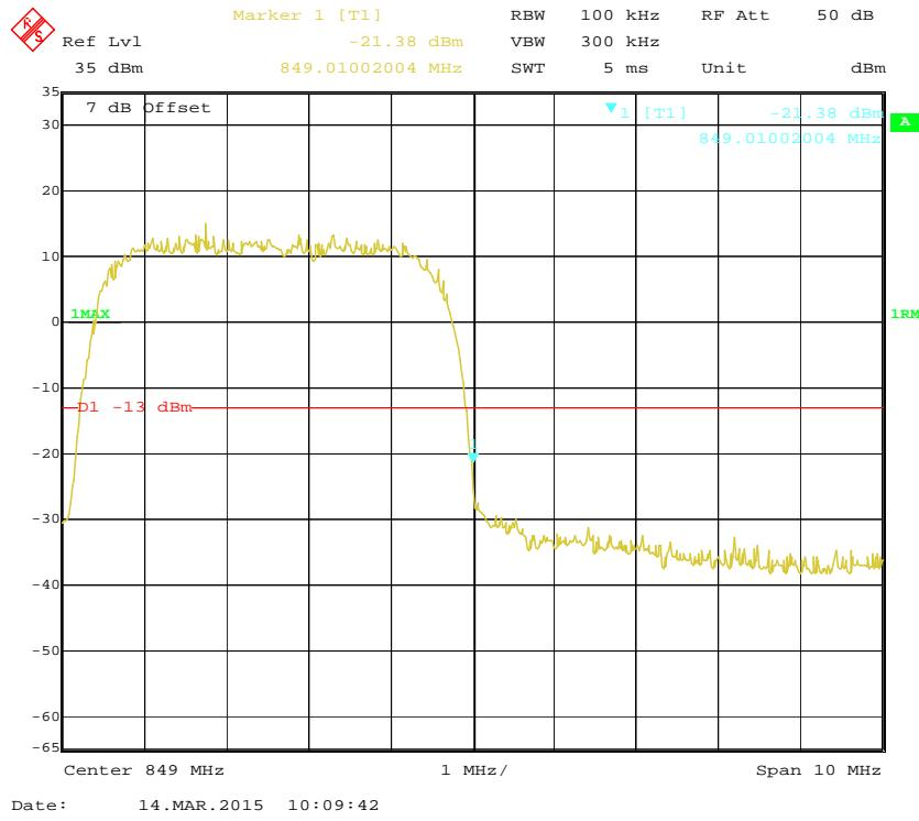
**PCS Band, Left Band Edge for GSM (GMSK) Mode**
