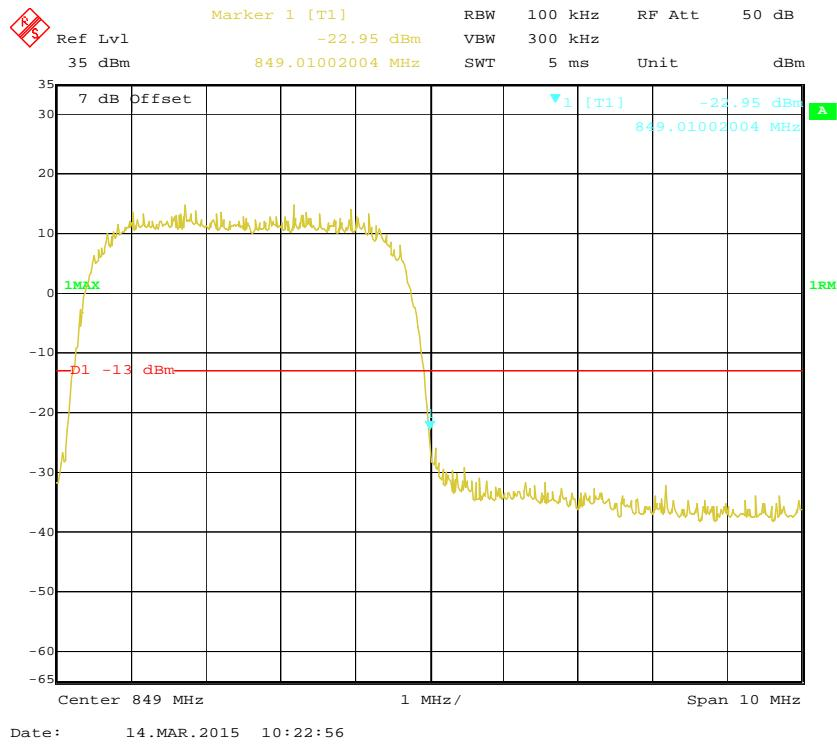
**Cellular Band, Left Band Edge for HSUPA (BPSK) Mode**
