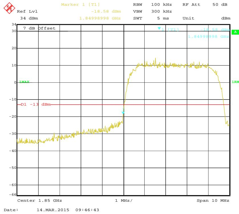
**PCS Band, Right Band Edge for HSUPA (BPSK) Mode**
