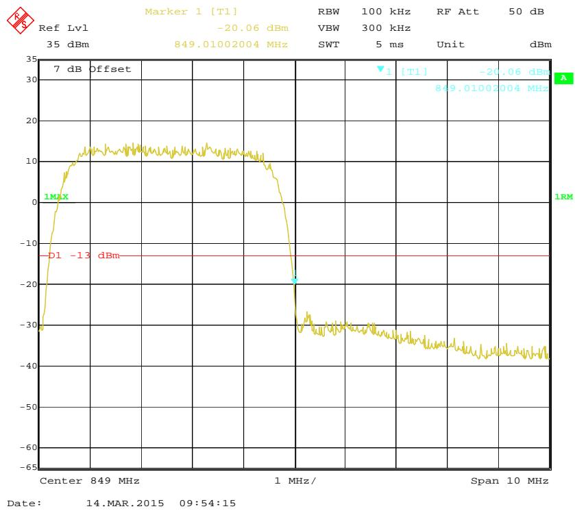
**Cellular Band, Left Band Edge for HSDPA (16QAM) Mode**
