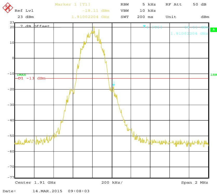
**PCS Band, Left Band Edge for WCDMA (BPSK) Mode**
