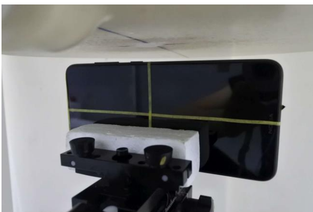
Right Side, Test Separation 10 mm
