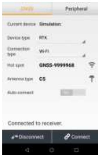
Tap the Wireless Lan icon on the right side to select the hot spot → Switch on the WiFi module by the top switch → select the target device in the list.
