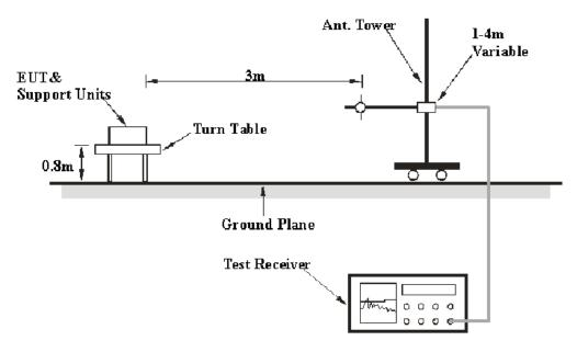
Note: Antenna is set up at 1m during test for below 30MHz.
