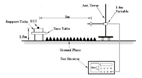
The radiated emission tests were performed in the 3 meters test site, using the setup accordance with the ANSI C63.10-2013. The specification used was the FCC 15.209, and FCC 15.247 limits.
