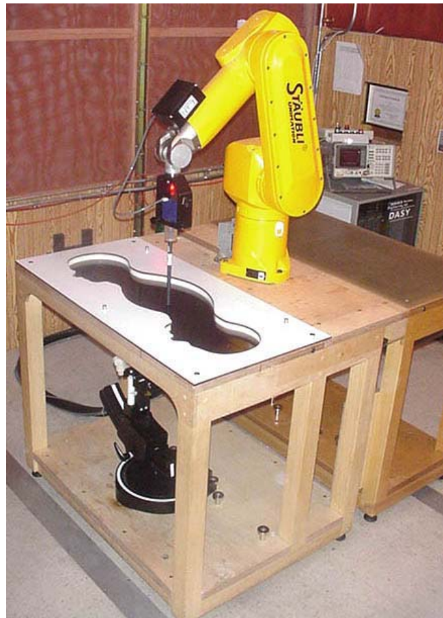
DASY4 Measurement System with SAM Phantom & 5GHz Fluid
