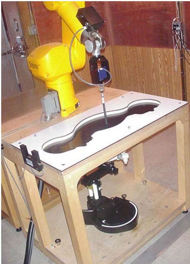
DASY4 SAR Measurement System with SAM phantom & 5GHz Fluid
