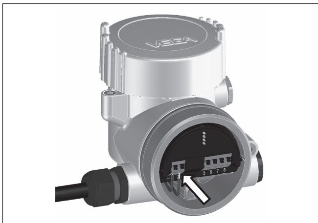
Fig. 24: Connection steps 5 and 6 - Double chamber housing
