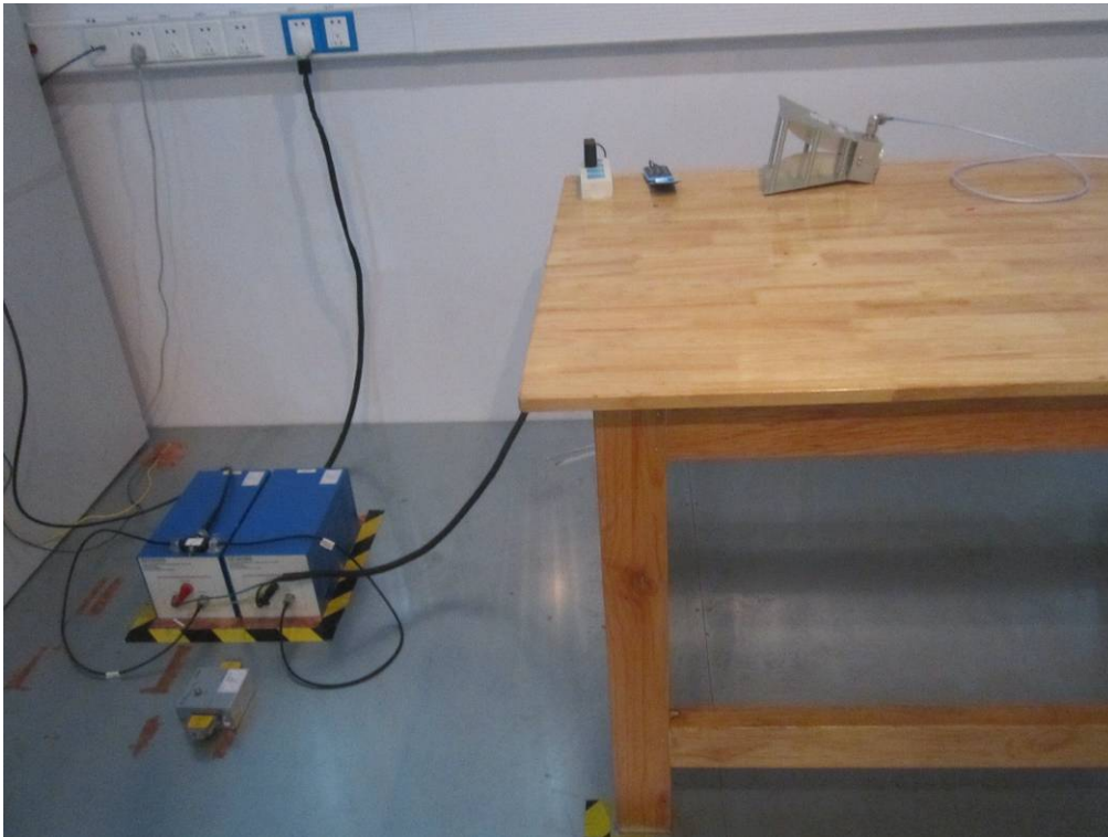
Conducted Emissions Test Setup Front View
