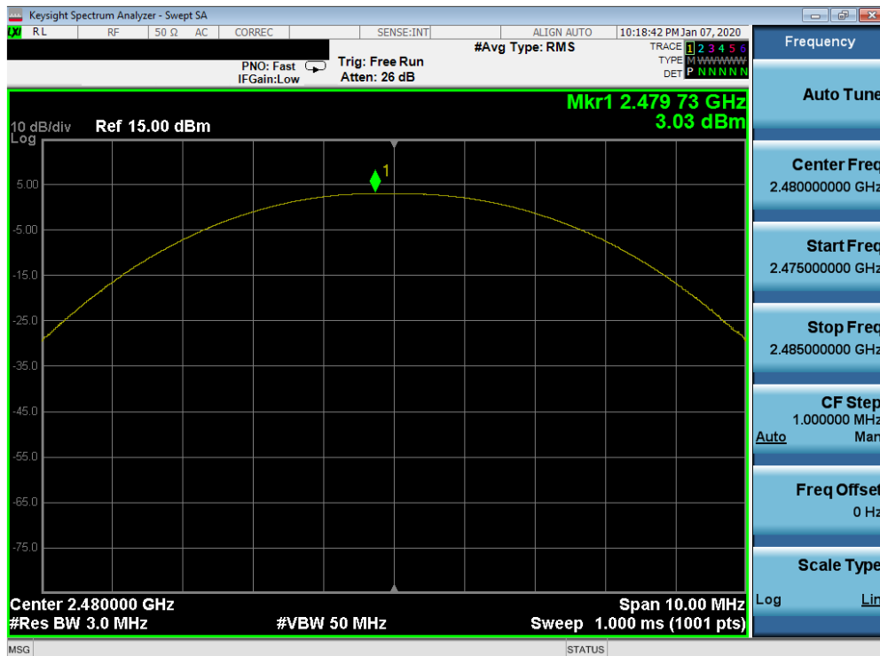
Plot 7-18. Peak Power Plot (Bluetooth (LE), 500kbps – Ch. 39)
