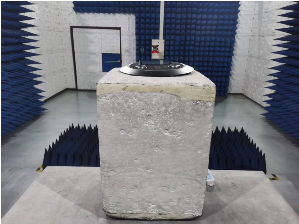
RADIATED EMISSION TEST SETUP ABOVE 1GHz
