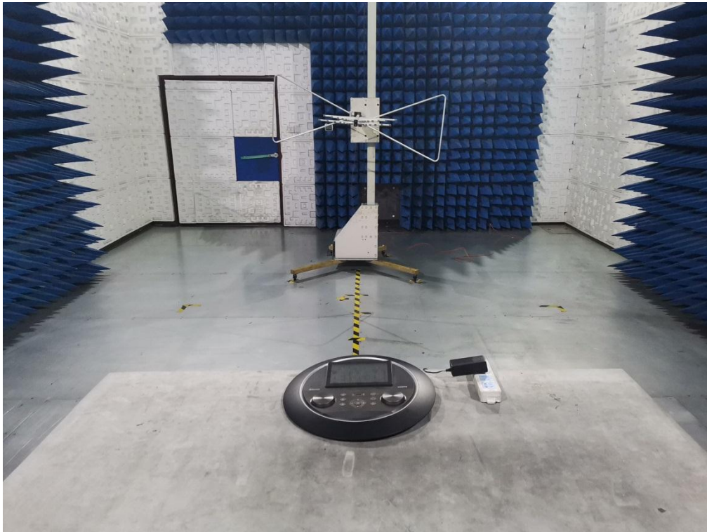
RADIATED EMISSION TEST SETUP ABOVE 1GHz
