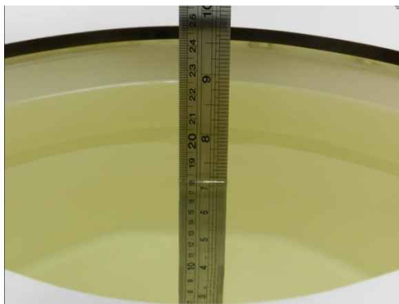
Fig 10.1 Photo of Liquid Height for Body SAR
