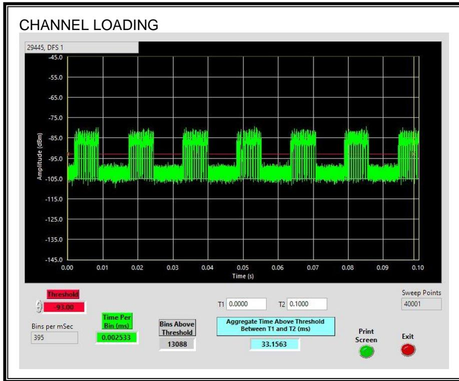
The level of traffic loading on the channel by the Master is 33.15%
