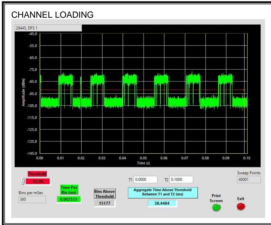
The level of traffic loading on the channel by the Master is 38.44%
