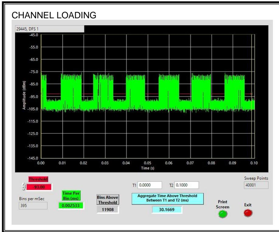
The level of traffic loading on the channel by the Master is 30.16%
