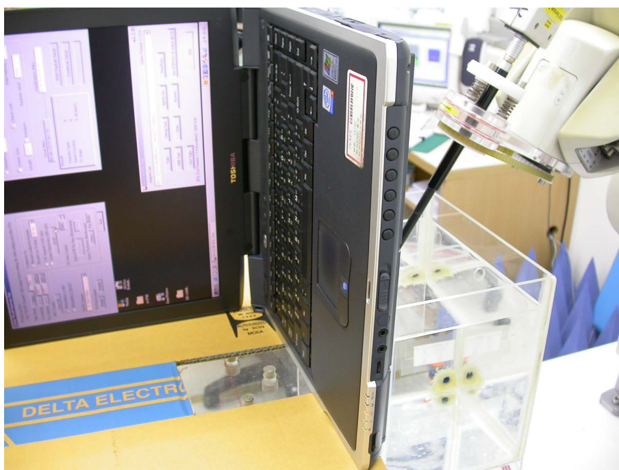
Figure 14: EUT bottom to phantom, 0 mm separation
