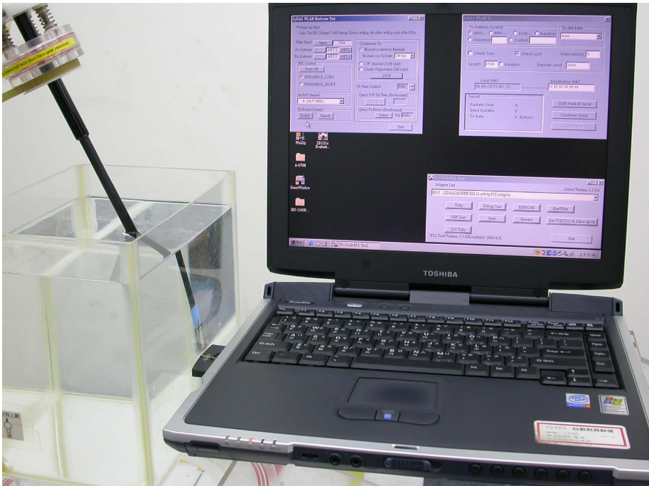
Figure 16: EUT perpendicular to phantom, 0 mm separation
