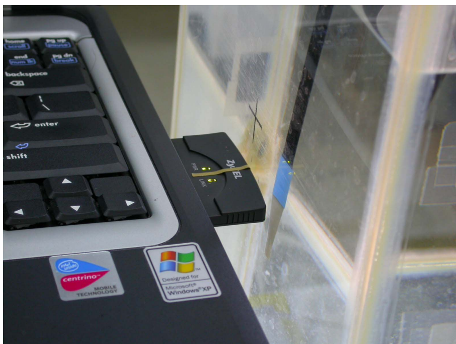
Figure 11: EUT perpendicular to phantom, 0 mm separation-Zoom in
