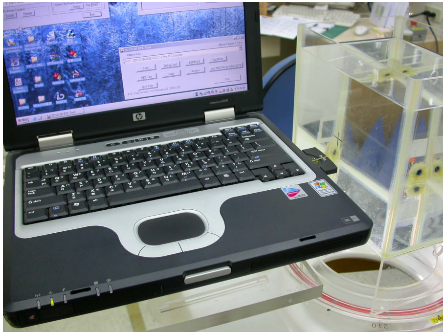
Figure 12: EUT perpendicular to phantom, 15 mm separation
