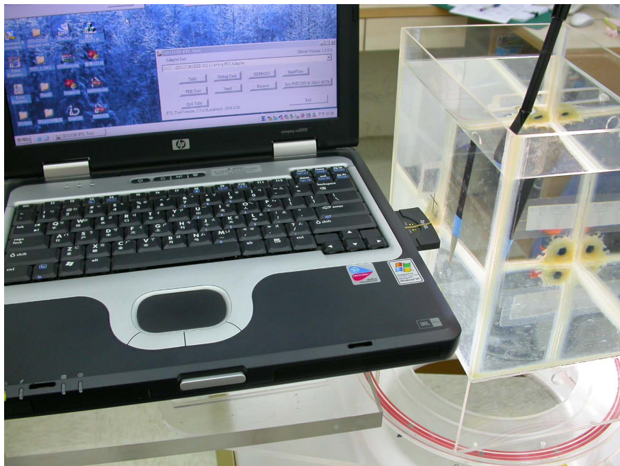
Figure 10: EUT perpendicular to phantom, 0 mm separation
