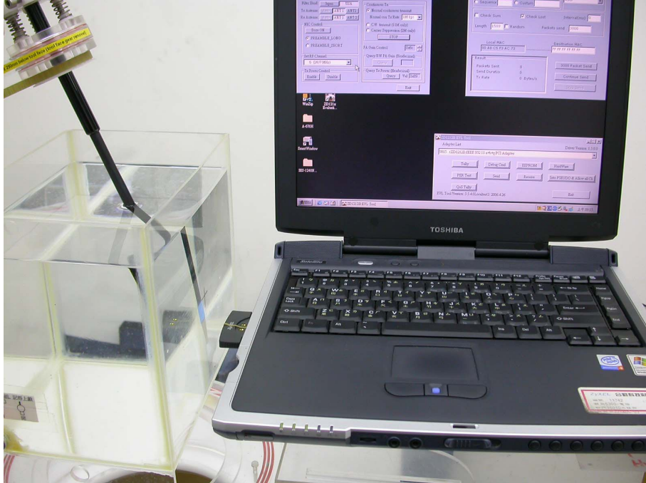
Figure 18: EUT perpendicular to phantom, 15 mm separation
