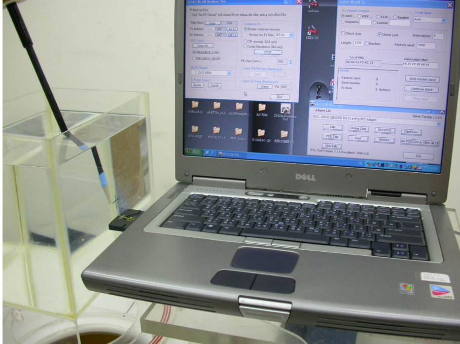
Figure 4: EUT perpendicular to phantom, 0 mm separation
