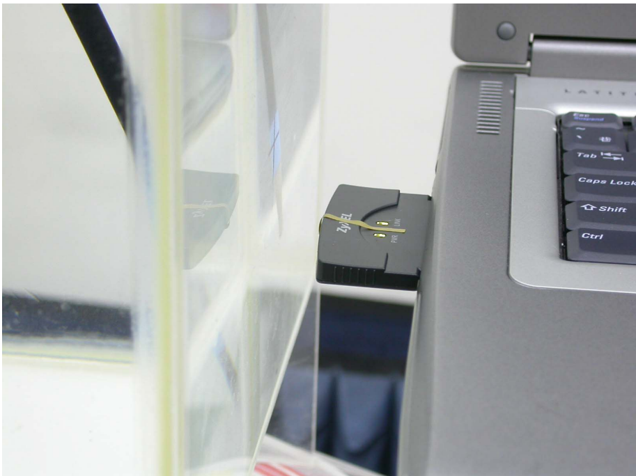
Figure 7: EUT perpendicular to phantom, 15 mm separation-Zoom in
