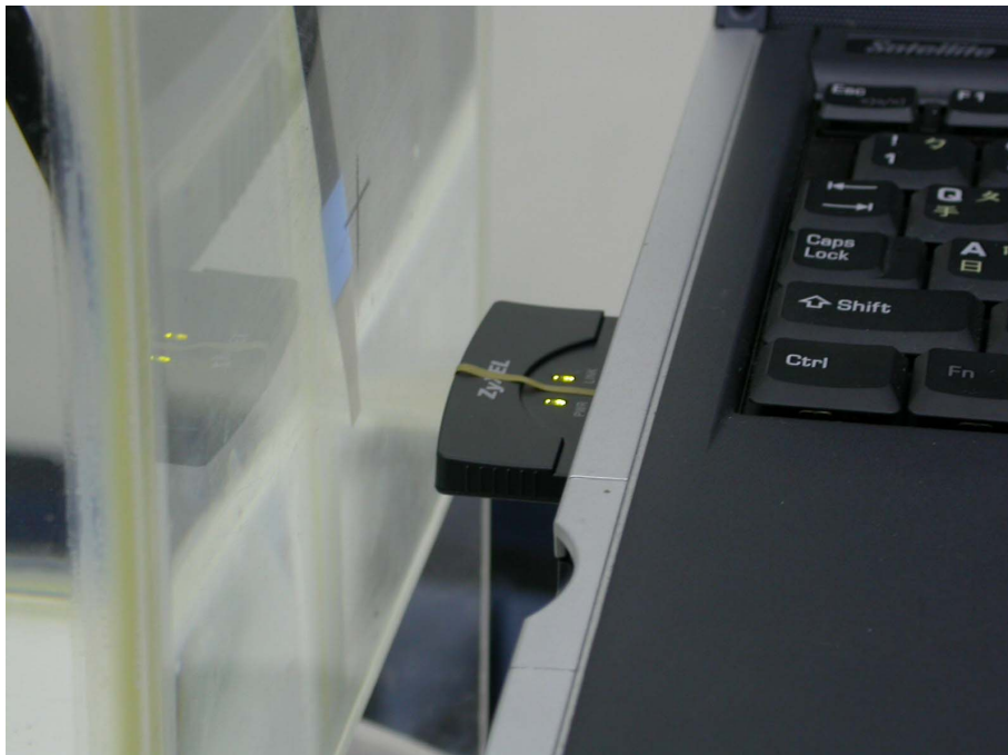
Figure 19: EUT perpendicular to phantom, 15 mm separation-Zoom in
