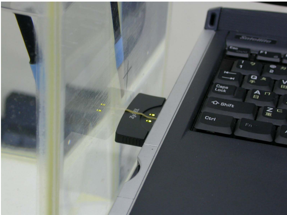
Figure 17: EUT perpendicular to phantom, 0 mm separation-Zoom in
