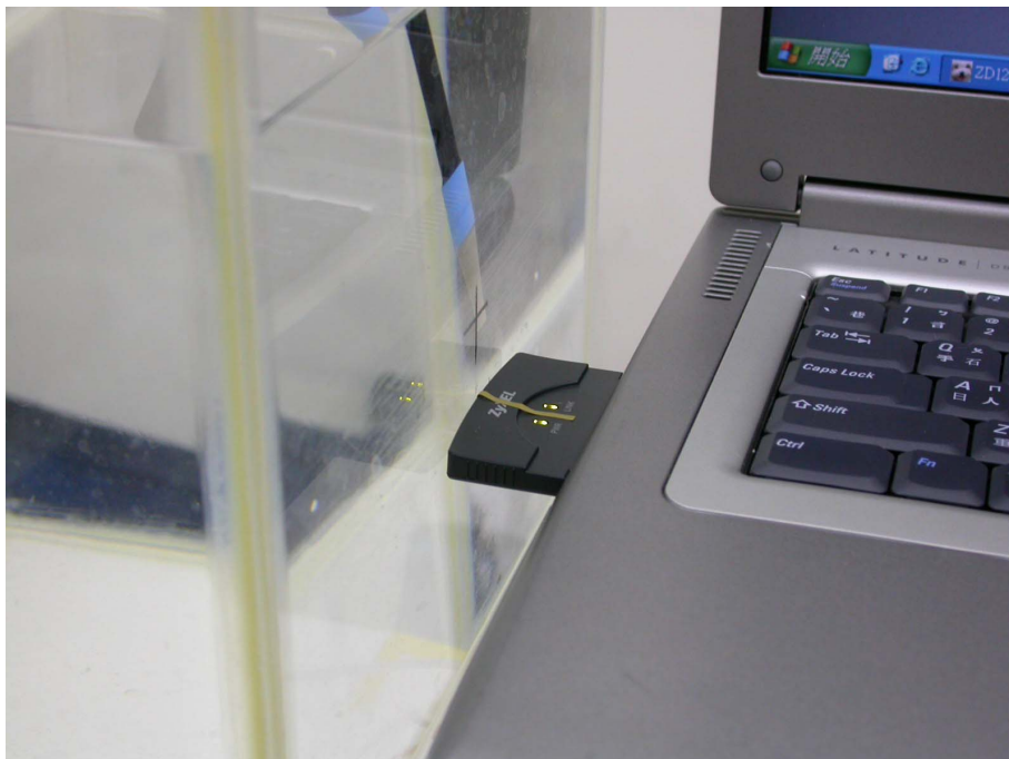
Figure 5: EUT perpendicular to phantom, 0 mm separation-Zoom in
