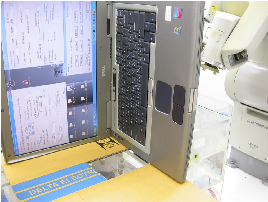
Figure 2: EUT bottom to phantom, 0 mm separation
