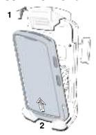
To remove the TC58 from the cradle, lift the release latch, grasp the TC58 and lift out of the vehicle cradle.
