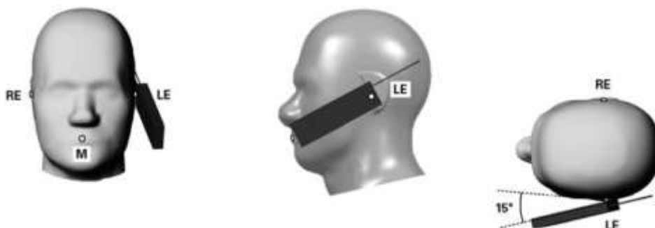
Figure 6.5. Tilt 15^\circ position of the wireless device
